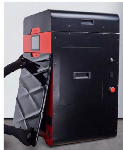
Image 61. Method of taking off the front panel.
