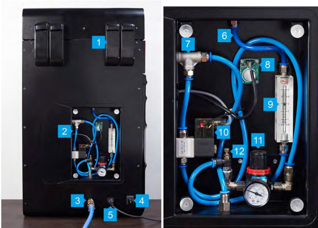
Image 3. View of the printer's gas installation.
