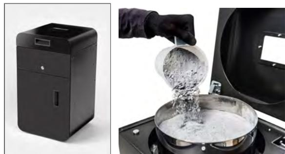
Image 54. Sieving the powder using Sinterit POWDER SIEVE.
