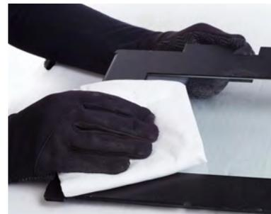
Image 15. Cleaning of LASER PROTECTIVE GLASS.
