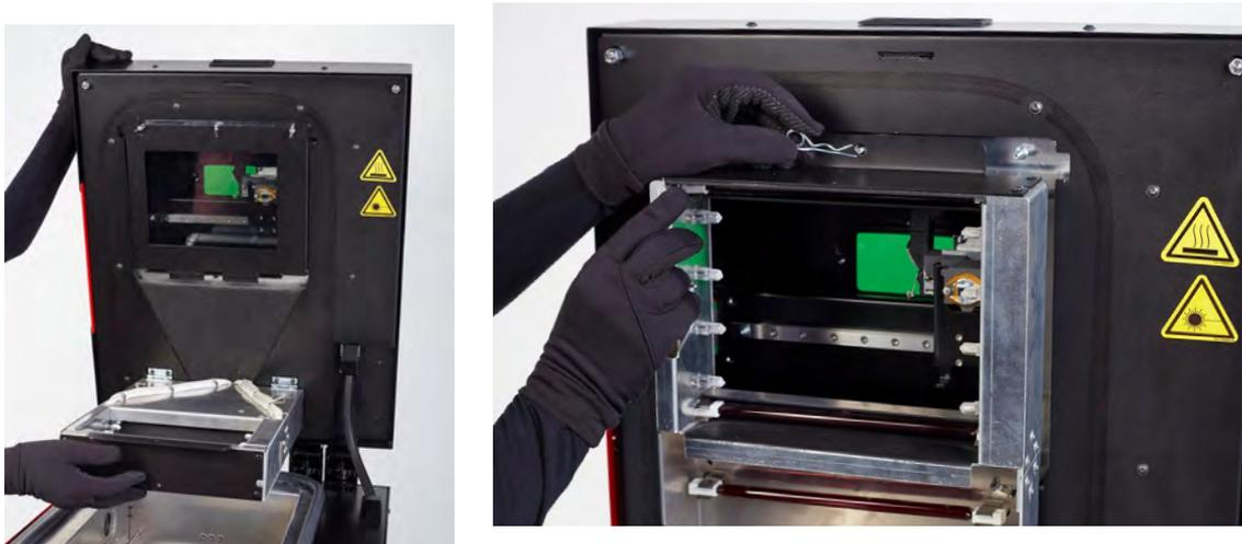
Image 17. Correct closing of the heating module.
