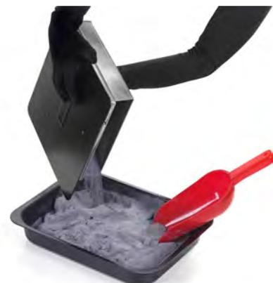
Image 41. Correct cleaning of the OVERFLOW BIN.
