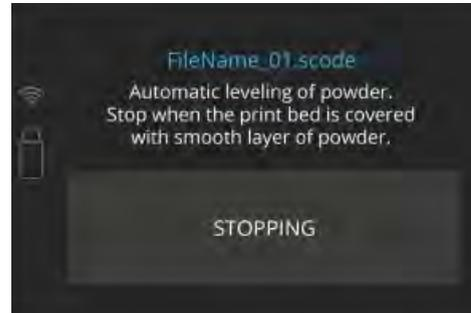
Image 30. Stopping the leveling process manually screen.
