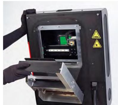
Image 13. Heater module - opening.
