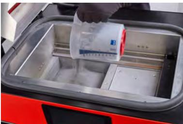
Image 25. Step 1. Adding powder to the FEED BED .
