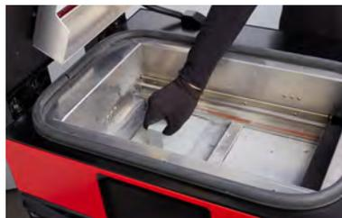
Image 26. Step 2. Compacting powder by gently pressing it.
