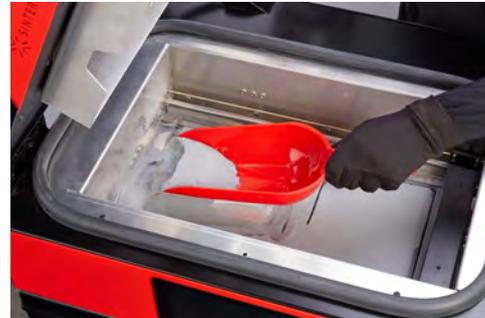
Image 45. Removing the powder from the FEED BED.
